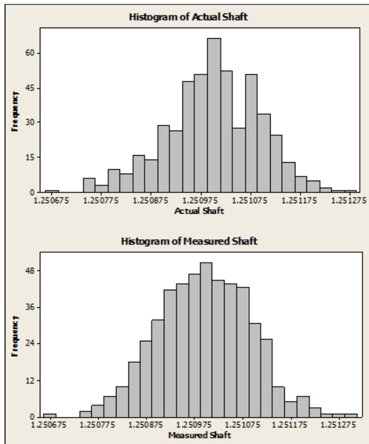
Figure 15 Comparison of Actual and Measured Shaft Diameters for On Target with Minimal Variation
