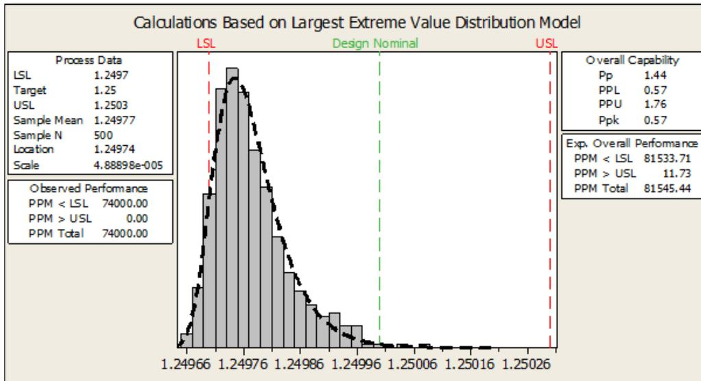
Figure 7 "Passed Bad" Misclassification Rates of Actual Bore Diameters for Max. Metal Machining
