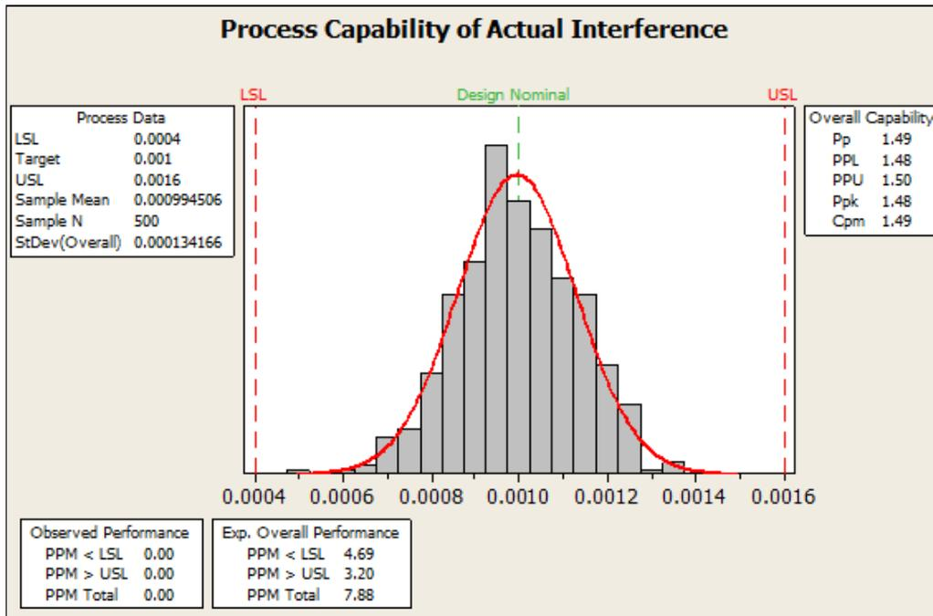
Figure 19 Process Capability of Actual Interference Fits for On Target with Minimal Variation
