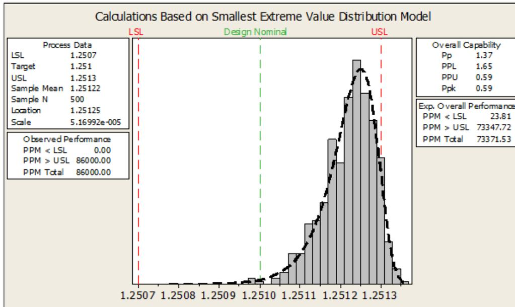
Figure 9 "Passed Bad" Misclassification of Actual Shaft Diameters for Max. Metal Machining
