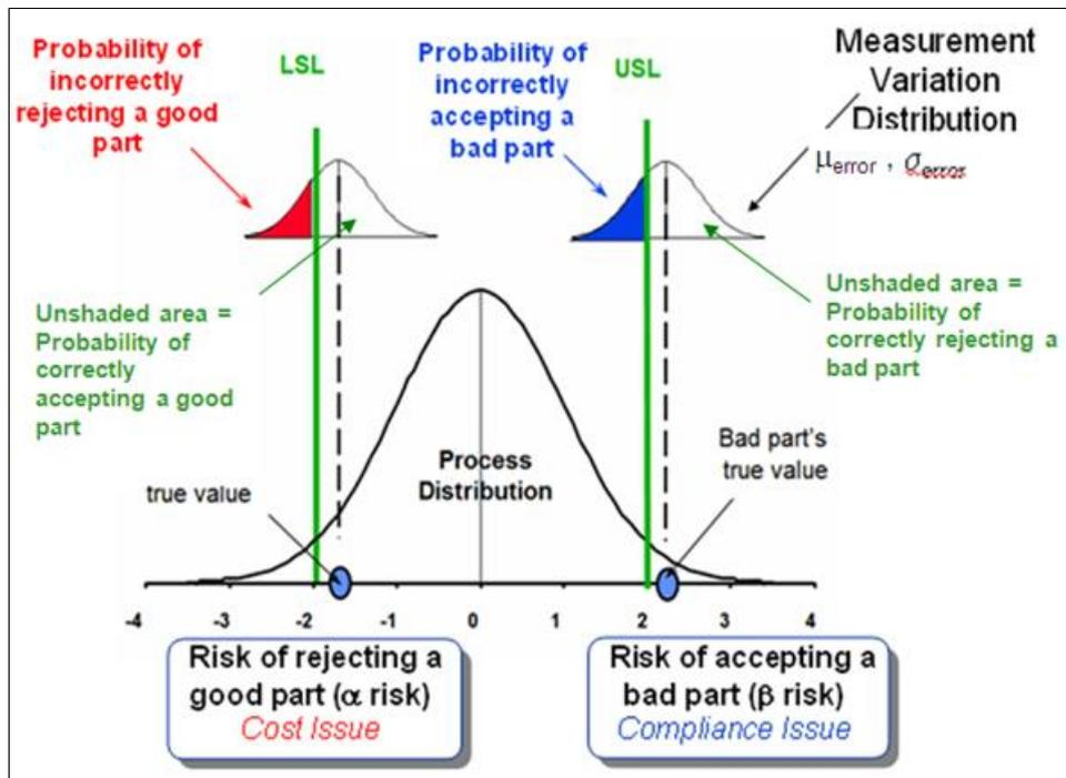
Figure 1 Classification and Misclassification of Parts due to Measurement System Variation
