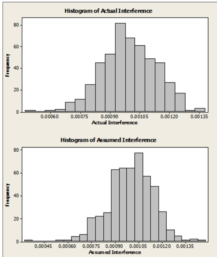
Figure 18 Comparison of Actual and Assumed Interference Fits for On Target with Minimal Variation
