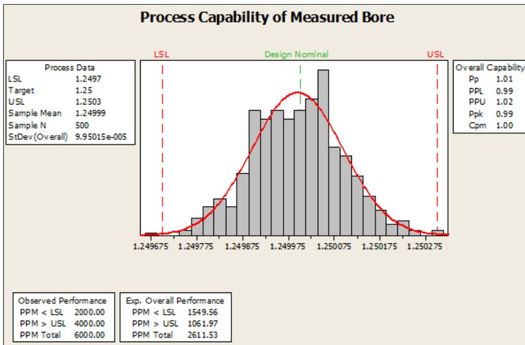
Figure 14 Process Capability of Measured Bore Diameter for On Target with Minimal Variation
