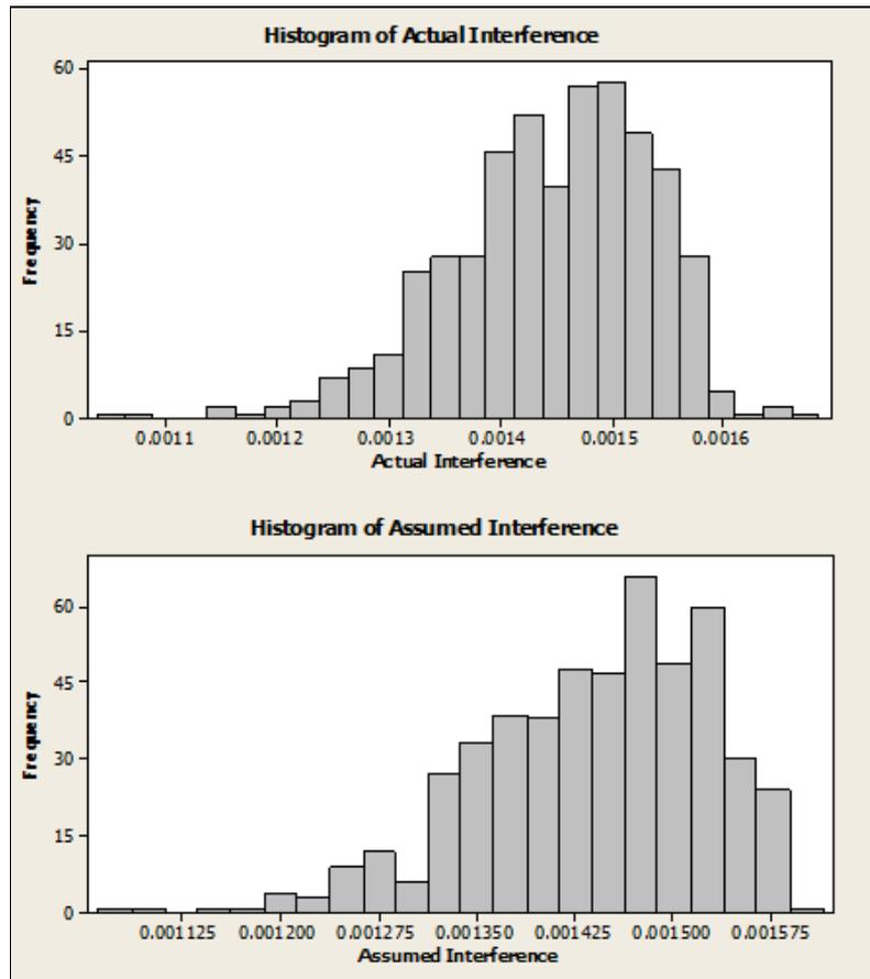
Figure 10 Comparison of Actual and Assumed Interference Fits for Max. Metal Machining
