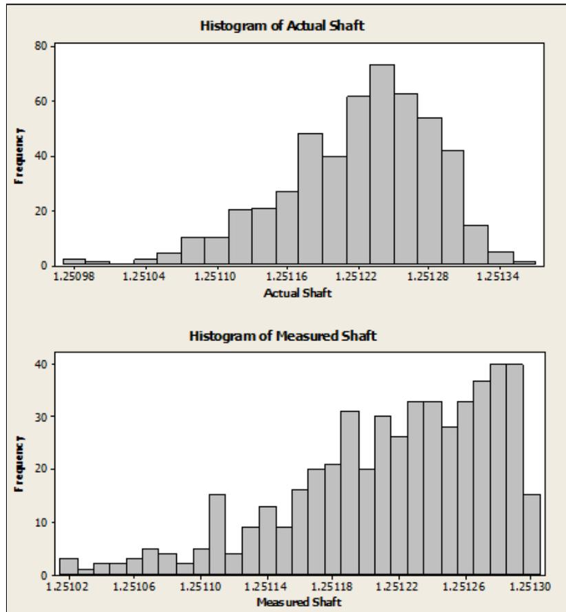
Figure 8 Comparison of Actual and Measured Shaft Diameters for Max. Metal Machining
