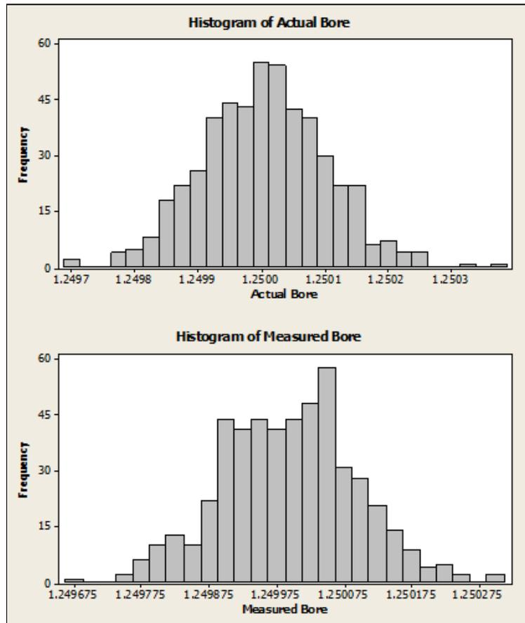
Figure 12 Comparison of Actual and Measured Bore Diameters for On Target with Minimal Variation
