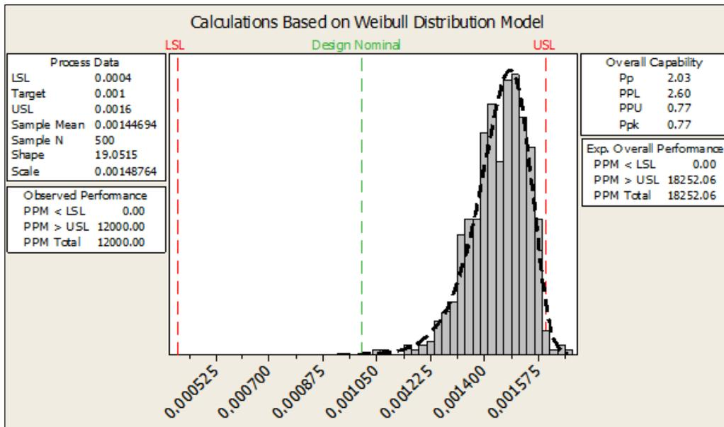
Figure 11 Process Capability of Actual Interference Fits for Max. Metal Machining
