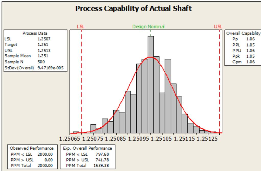
Figure 16 Process Capability of Actual Shaft Diameter for On Target with Minimal Variation
