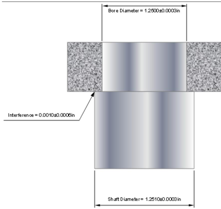
Figure 5 Bore and Shaft Assembly to an Interference Fit
