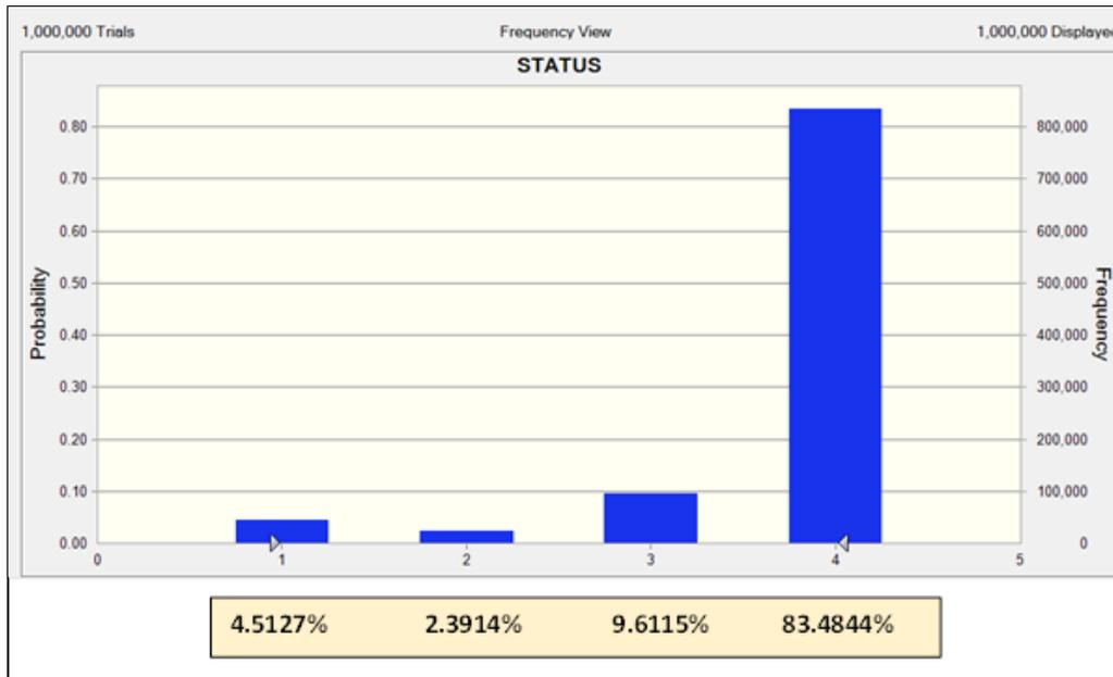
Figure 2 Classification and Misclassification of Parts from Monte Carlo Simulation
