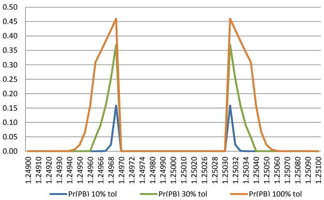
Figure 4 Probability of Passing Bad Parts versus True Bore Diameter
