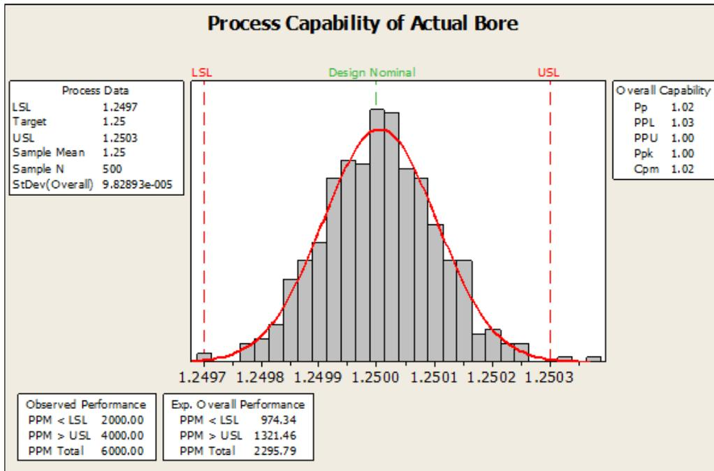
Figure 13 Process Capability of Actual Bore Diameter for On Target with Minimal Variation
