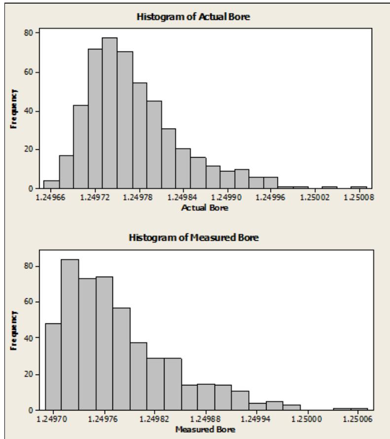
Figure 6 Comparison of Actual and Measured Bore Diameters for MMM
