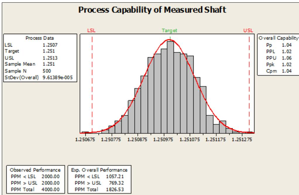
Figure 17 Process Capability of Measured Shaft Diameter for On Target with Minimal Variation
